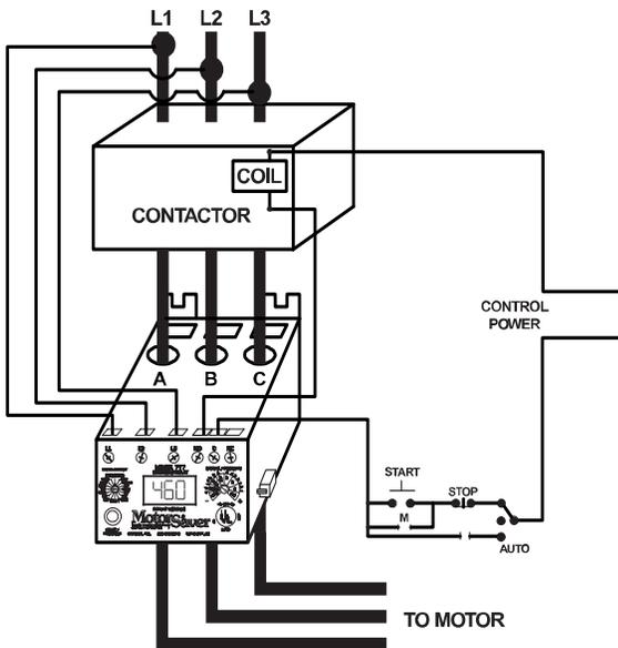
CURRENT TRANSFORMER WIRING DIAGRAM FOR MODEL 777 (80 TO 800 AMPS)
